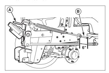
Figure 24. Lift Spring Assist Crank
